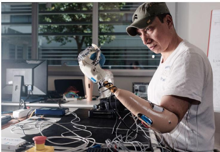
Figure. During their master's final project, students were asked to develop and clinically evaluate a neuro-controlled upper limb prosthesis intuitively controlled and felt by the amputee as the natural one (courtesy of Silvestro Micera's lab, EPFL).
