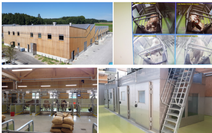
Fig. 2. Metabolic Center of AgroVet-Strickhof. Top left: building; bottom left: facility for balance experiments; top right: respiration chambers stocked with dairy cows; bottom right: outside view of four medium-sized respiration chambers.
